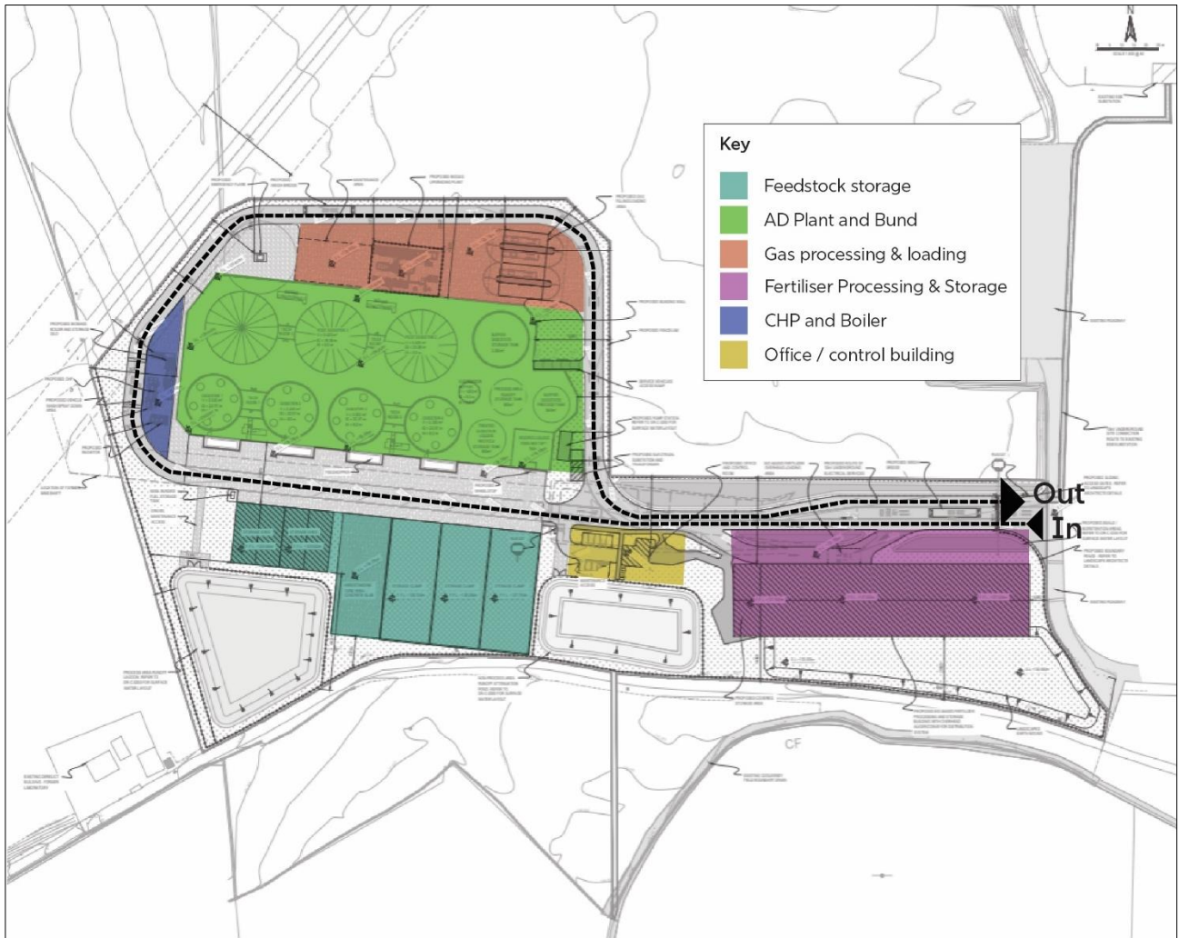
Figure 6.1: Overview of the Proposed Site Layout. Source: Extract of Drawing No. 2429-DOB-XX-SI-DR-C-0500 P01, annotated by Purser to show key zones within the proposed site layout.
